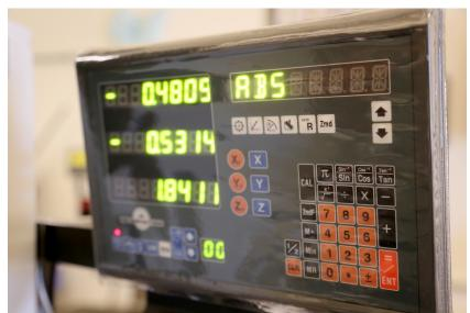
A digital readout displays the movement of the x- and y-coordinate system on a geared milling and drilling machine inside Butler County Community College's manufacturing lab on Monday, July 15, 2019.
